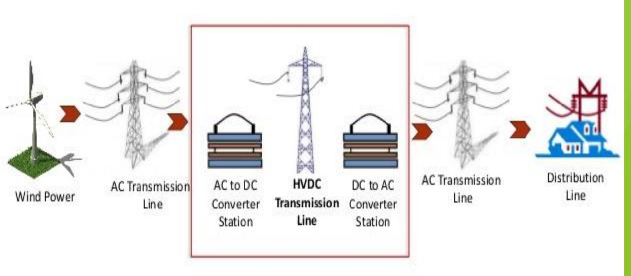
Components of an HVDC transmission system
